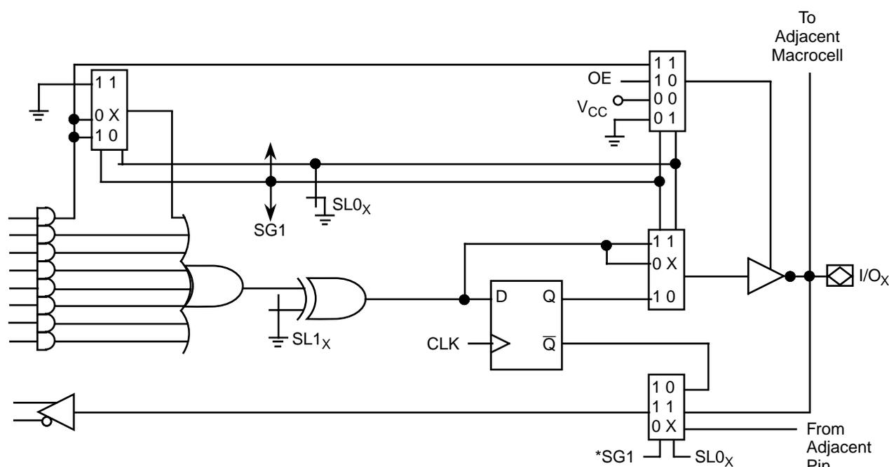
\*In macrocells MC<sub>0</sub> and MC<sub>7</sub>, SG1 is replaced by  $\overline{SG0}$  on the feedback multiplexer.
